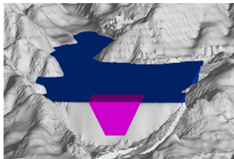
Fig. 12 Trapezoidal moving object image defined in the numerical model
