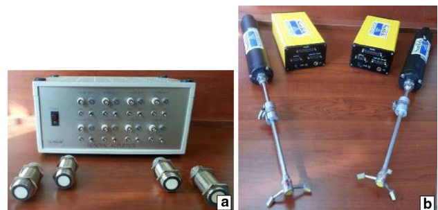
Fig. 3 a ULS 80-D device and USS20130 sensors; b MicroADV device and probes
