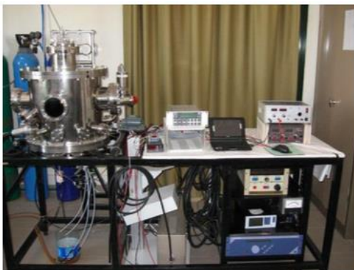
Figure 19. Photograph of the magnetic field sputtering system in the infrastructure of the RACQUT.
