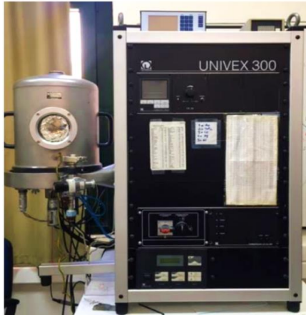
Figure 18. Photograph of the physical deposition system (PVD) (Leybold Univex 300) in the infrastructure of the Research and Application Center for Quantum Technologies (RACQUT).
