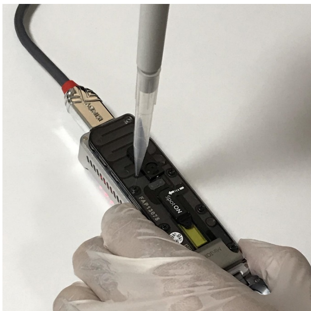
Figure 9. MinION flow cell priming
