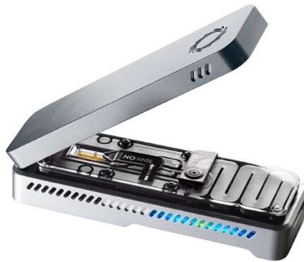
Figure 6. The Oxford Nanopore Technologies MinION sequencer (Source: Oxford Nanopore Technologies, 2022)
