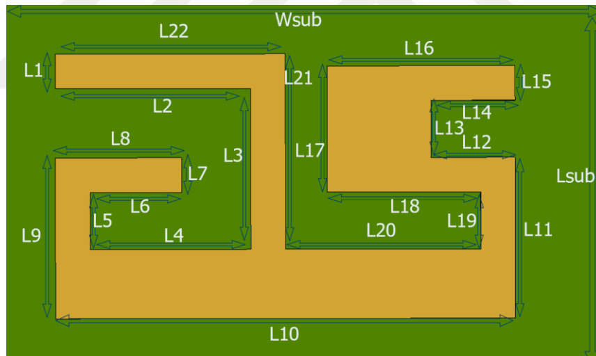
Figure 7. The proposed G&S MMA design with the design parameters.
