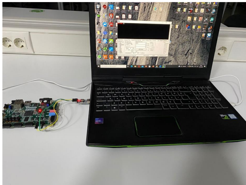
Figure 30. Real-time data acquisition through UART communication
