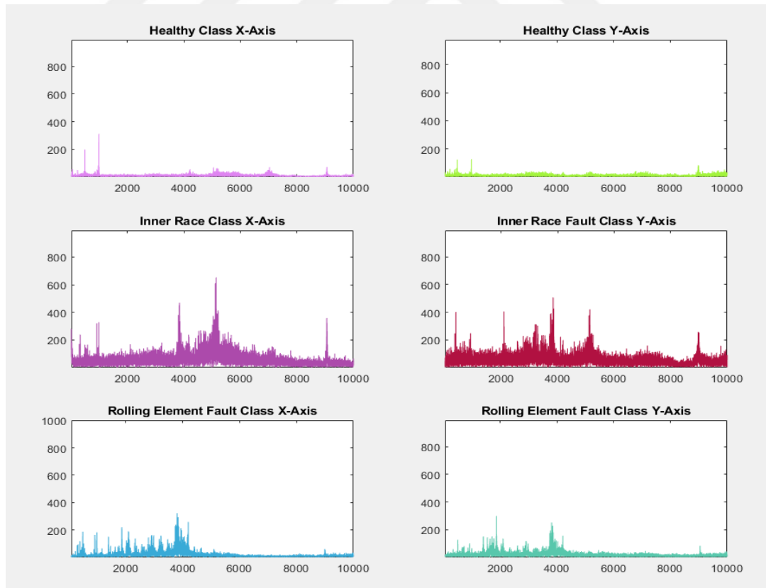
Figure 23. Corresponding vibration signals in Fourier Domain for healthy state and inner race fault cases of x -axis and y -axis from IMS Bearing Dataset.
