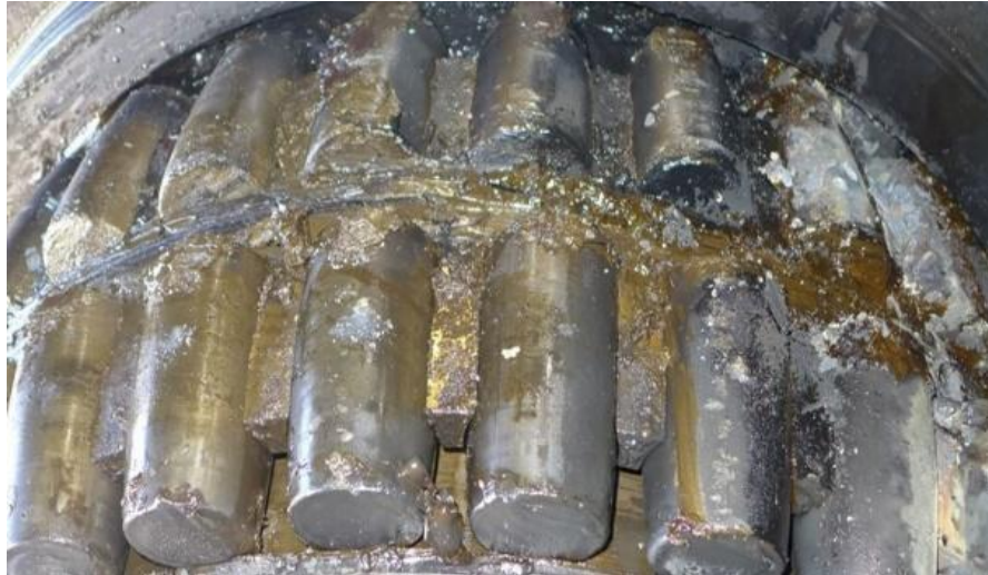
Figure 5. Typical real lubrication failure (Source: Micro-Lube, 2021).
