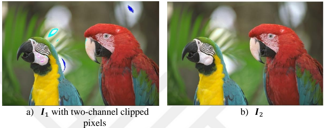
Figure 4. Two-Channel Correction: (a) \{R, G\} , \{R, B\} and \{G, B\} Jointly Clipped Pixels are represented in Cyan, Magenta and Dark Blue, Respectively; (b) Two-Channel Corrected Output Image I_2 .
