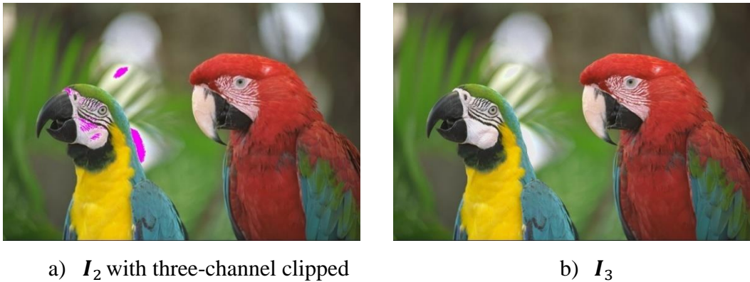
Figure 6. Three-Channel Correction: (a) Pixels clipped in all Channels are represented in Magenta and (b) Three-Channel corrected Output Image I_3 .
