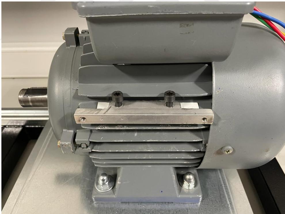
Figure 35. Aluminum mounting bracket.
