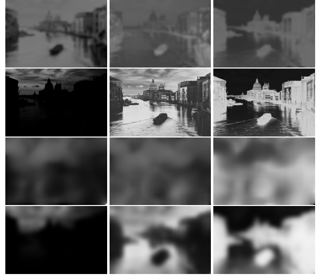
Fig. 2: Weights for Venice . (Top-to-bottom) PCA maps, adaptive well-exposedness weights, saliency maps, final fusion weights.
