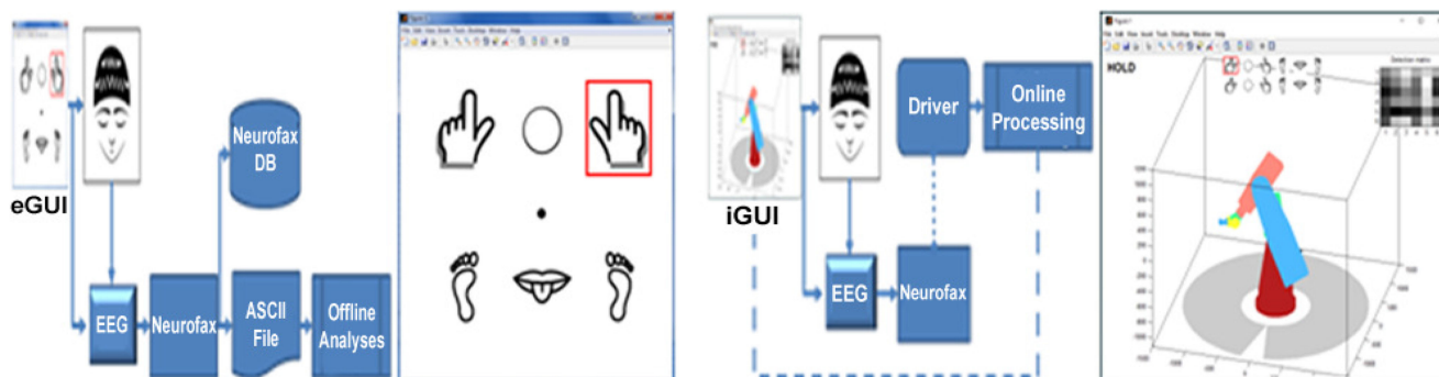
Fig. 1. (Left) Schematic representation of the offline experiments' procedure with experimental graphical user interface (eGUI). First, action signals had been presented to participants by indicating one of the motor imagery icons using a red rectangle on computer screen. The EEG signal in response to the implementation of shown motor imagery was acquired by EEG-1200 system and recorded using Neurofax software. After the completion of the experiment, the recorded EEG data was saved to Neurofax database as well as exported to an ASCII file for further custom offline processing. The graphical user interface used in offline experiment consisting of a single Matlab figure with 5 icons representing left hand, right hand, left leg, right leg, and tongue motor imageries, a passive signal indicated with a circle, a fixation point in the center, and an action signal shown as a red rectangle around right hand motor imagery icons. (Right) Schematic representation of the online experiments' procedure with interactive graphical user interface (iGUI). The participants attempted to control in real time a 3 dof robotic manipulator arm using the EEG BCI by implementing different motor imageries. The row EEG signal associated with implementation of each imagery was recorded by EEG-1200 system and imported to Matlab via custom memory-scanning driver software. The EEG data was then processed in a Matlab application and used to provide control signal for the robot arm. The online experiment's interactive graphical user interface (iGUI) consisting of a Matlab figure modeling in 3D the motion of a robot manipulator arm.
