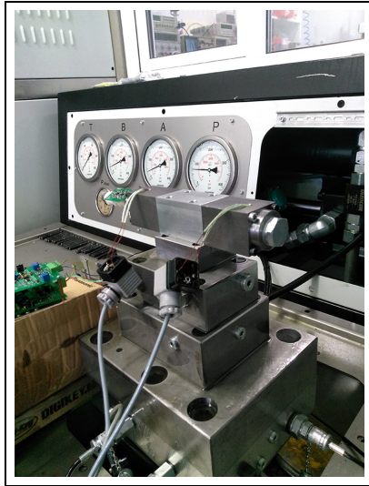
Figure 10. The manufactured solenoid with the optimized parameters along with the experimental setup.
