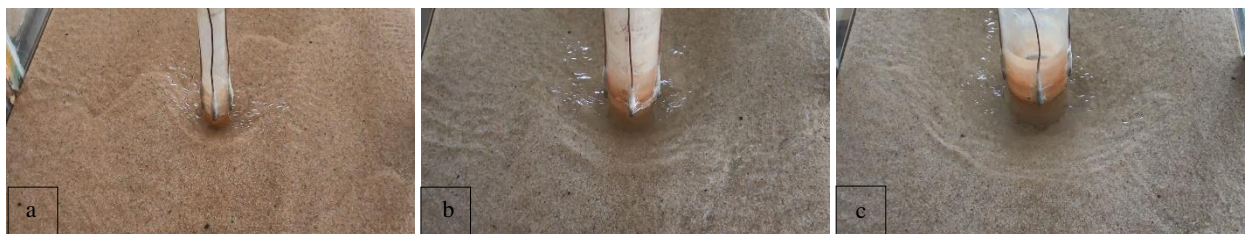
Figure 4. Scour holes at the end of the Hid55-38 for the pier a) D4; b) D8; and c) D11
