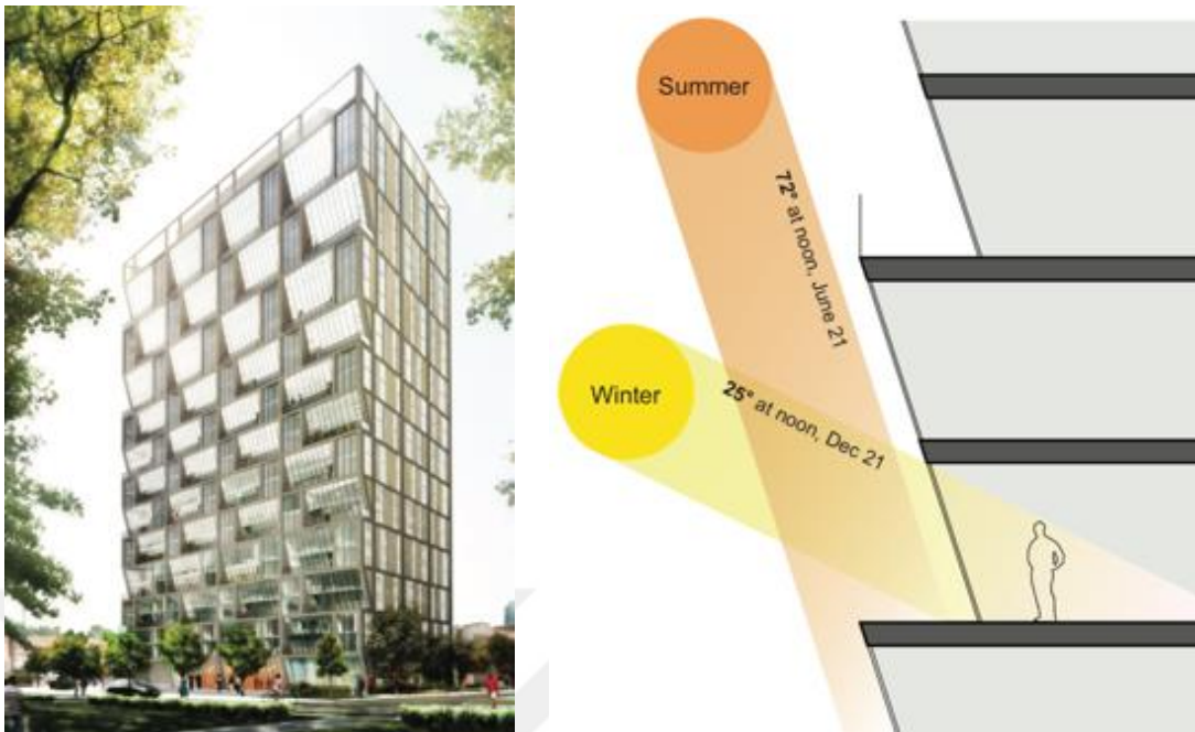
Figure 17. Left; Solstice on the Park designed by Jeanne Gang in Chicago in 2018. Right; inclined façade section located on the South façade. (Source: Oldfield, 2019)
