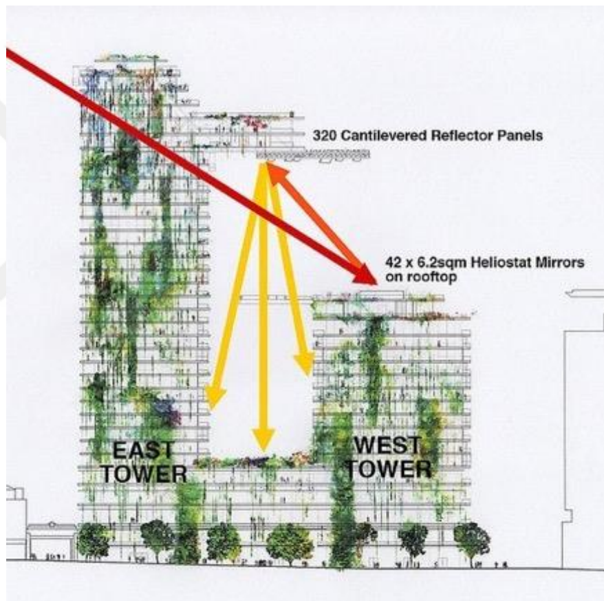
Figure 32. Top: Heliostats - Mirror Reflectors by Murray Fredericks. Bottom: Long Section of One Central Park. (Source: top; YeşilOdak, 2022 bottom; Modernist Architecture, 2013)
