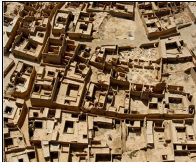
Figure 48. A layout of traditional Saudi houses showing courtyards in every house (Source: Al Surf et al., 2012)
