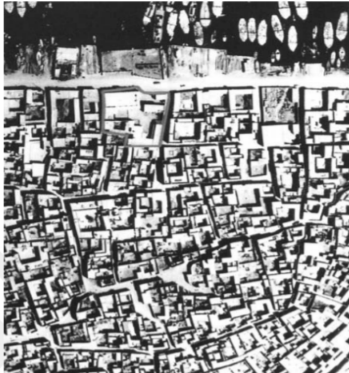
Figure 120. The arial view of Kuwait from the 1950's indicating the plot arrangements, with buildings placed adjacent to one another with narrow alleyways and each with the courtyards within the plot boundaries. (Source: Al-Beeshi et al.,2010)
