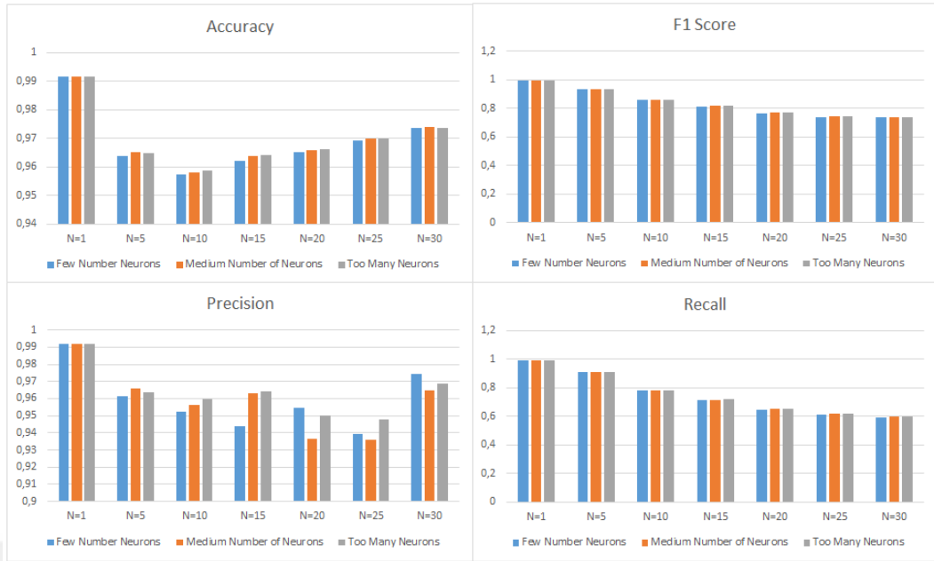
Figure 7.4: The Evaluation Scores of Convolutional Neural Network with Different Number of Neurons
