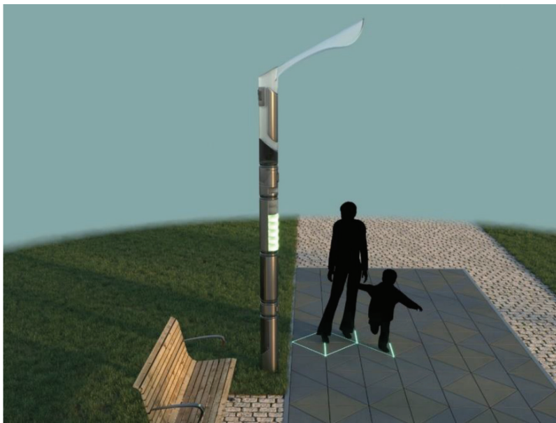
Figure 9: BAILIFF 2.0 improves user's awareness through gradual power indicator located in the product body.
