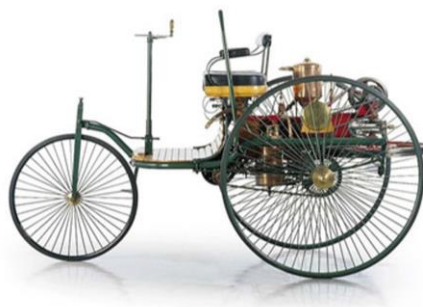
Figure 1. The first vehicle built by Carl Benz in 1886 (Source: Knoll, 2014)
