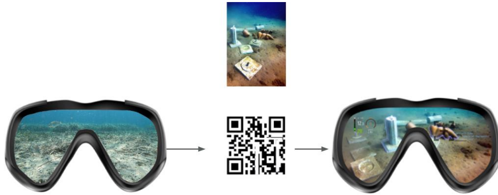
Figure 25- AR embedded diving mask system.
