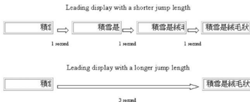
Figure 15. Example of two leading displays with the same speed but different jump length settings (Source: Wang, Fang, and Chen, 2003)
