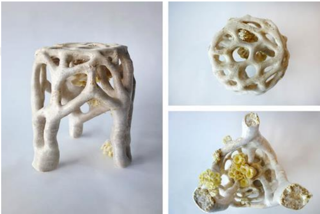
Figure 18-The “Veiled Lady 1.0” stool demonstrates an integration of a 3D-printed casing within which rigid volumes contain mycelium (Source: Myers, 2018)
