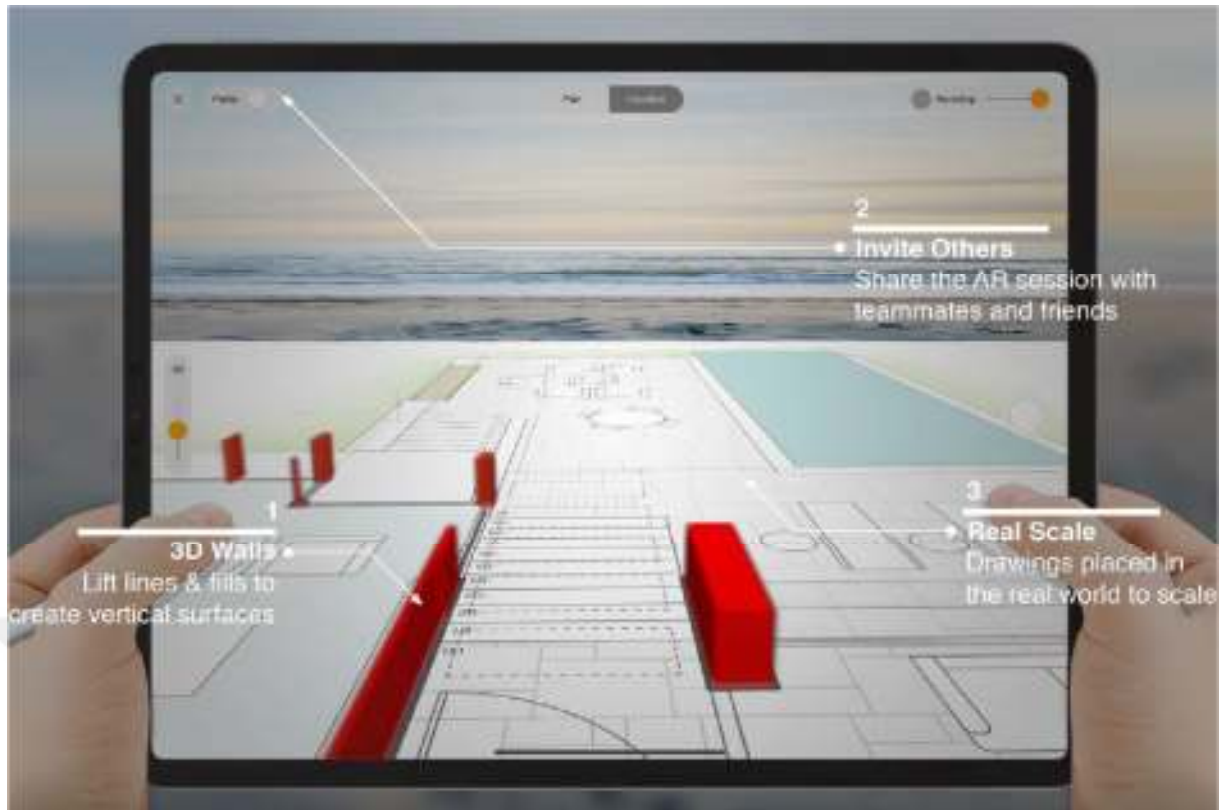
Figure 4.7. AR Sketchwalk Interior Architectural/Design Application Example (nbww, 2019).
