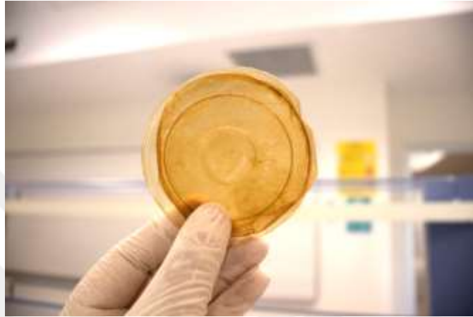
Figure 8. Bacterial cellulose biofilm (49,2% moisture)
