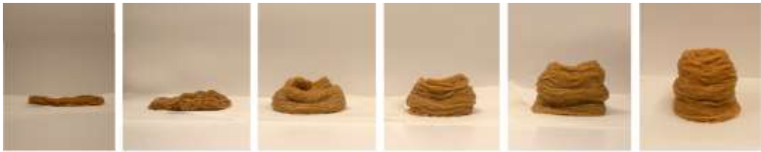
Figure 62. Enhanced structural integrity by creating matrices with fillers and gelling agents
