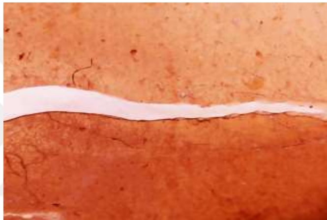
Figure 11. Dehydrated bacterial cellulose biofilm (0% moisture), cracked under tension x500
