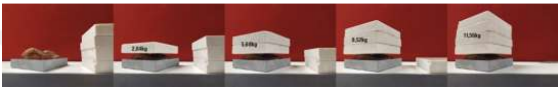
Figure 15. Analog bending test for BC-jute composite sample
