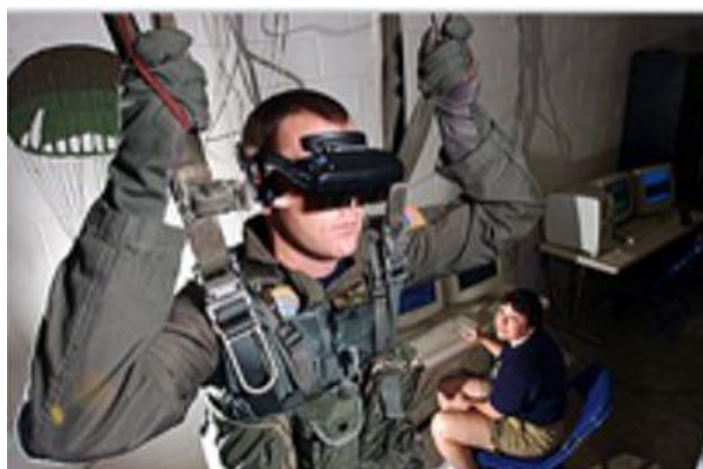
Figure 3.13 A VR parachute simulator demonstrated by US Navy medic at the Naval Survival Training Institute (Source: Wikiwand, 2019)
