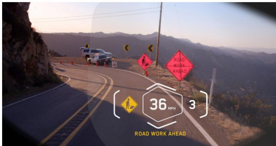
Figure 3.18 That is the HUD view propose of BMW's smart helmet design (Source: Canada Moto Guide, 2019)
