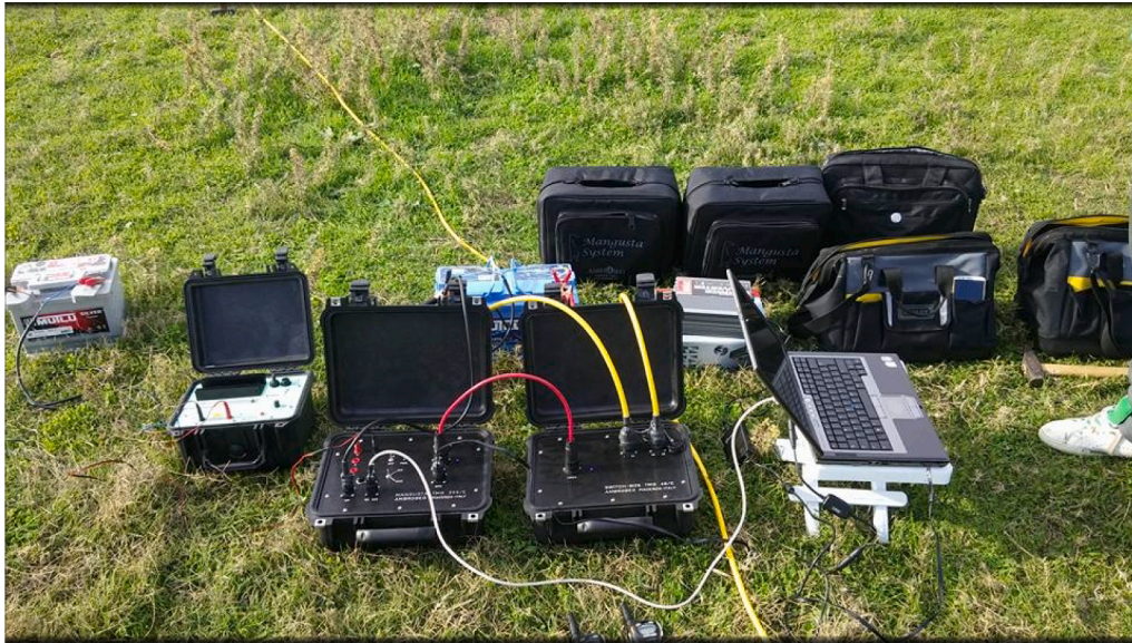
Fig. 16. Ambergeor brand's Mangusta TMG 255 E model multi-electrode (48 electrode capacity) resistivity tomography device.
