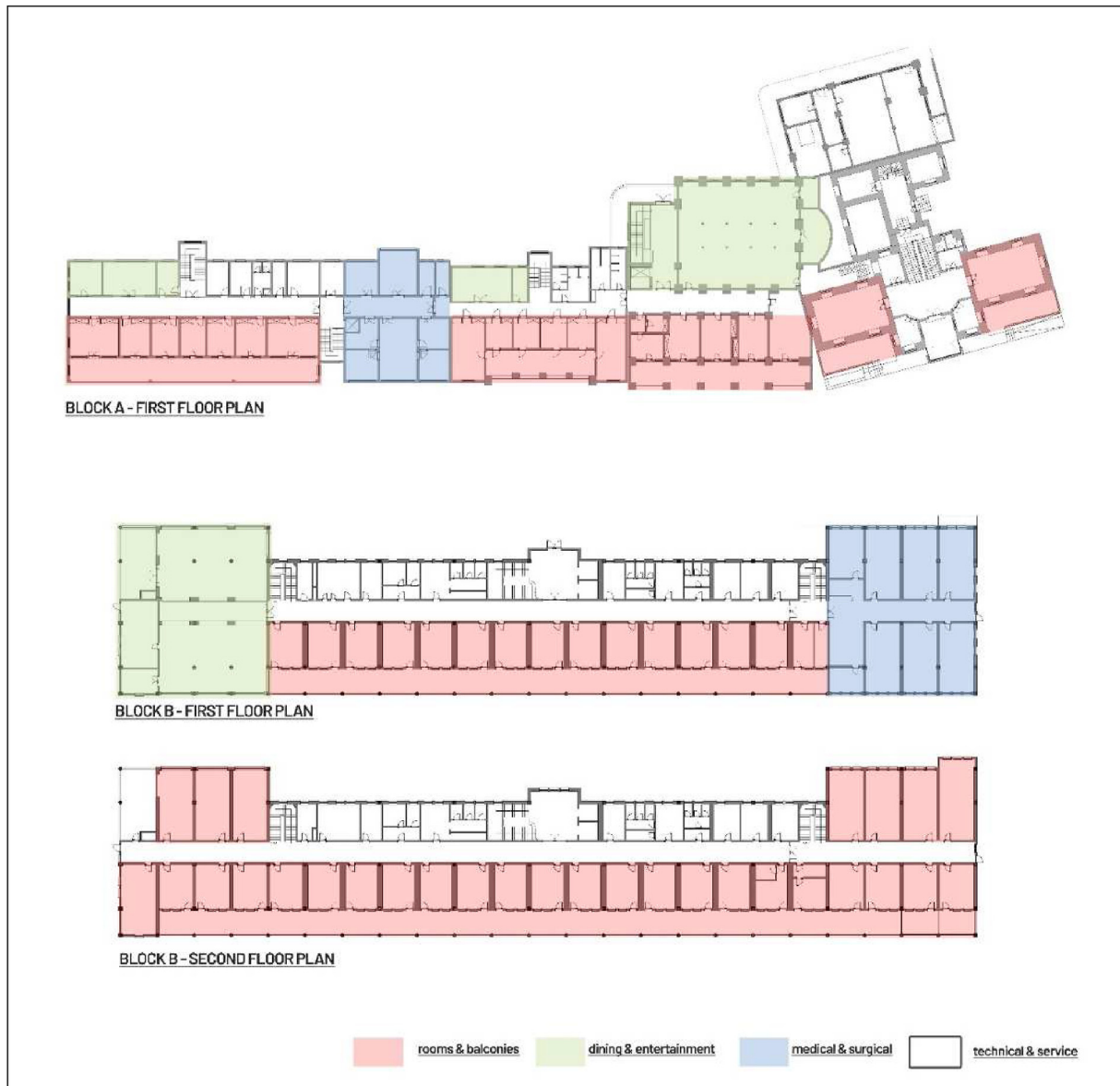
Fig. 26 The comparison of the spatial arrangement of Block A (1924–1945) and Block B (1945). Source: Courtesy of The Authors.
