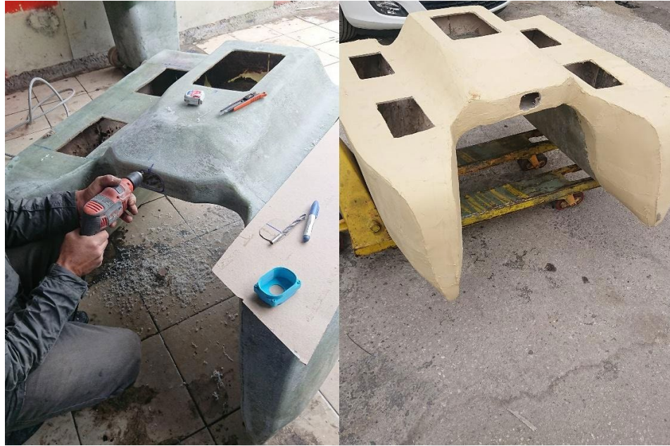
Figure 37. Glass fiber and Putty coating process
