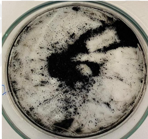
Figure 9. Synthesized magnetic particles for harvesting
