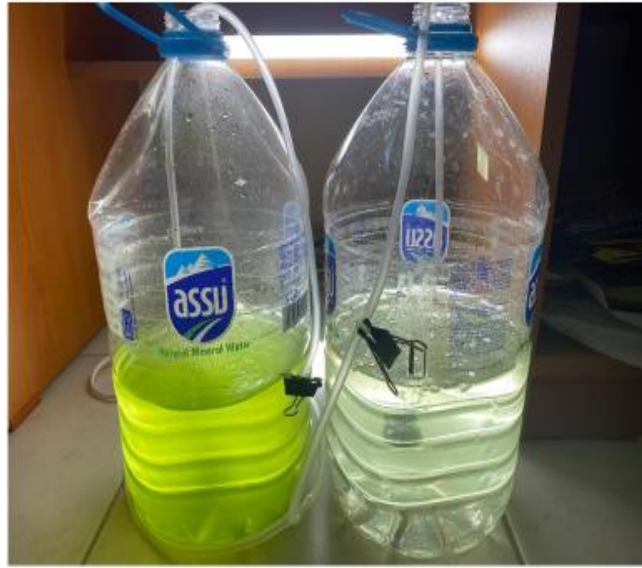
Figure 7. Microalgae cultivation without sterilization conditions. The first day of the cultivation appears on the right side and the last day on the left side.
