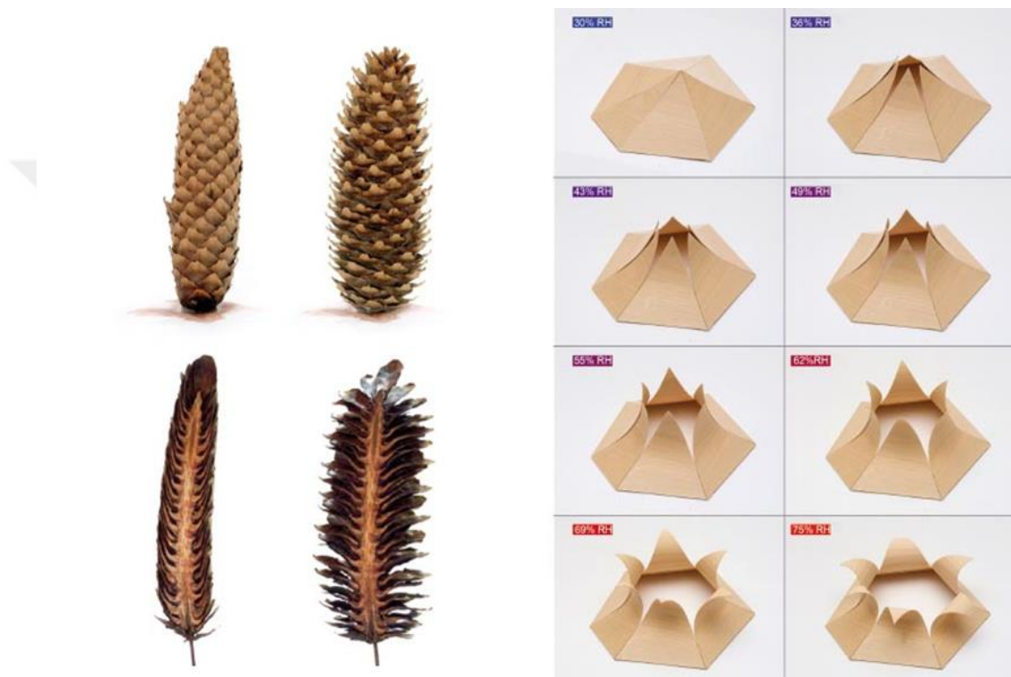
Figure 9. Transfer of the biological principle of shape change induced by hygroscopic and anisotropic dimensional change of the spruce cone (Source: Olivier Scheffer, 2016)
