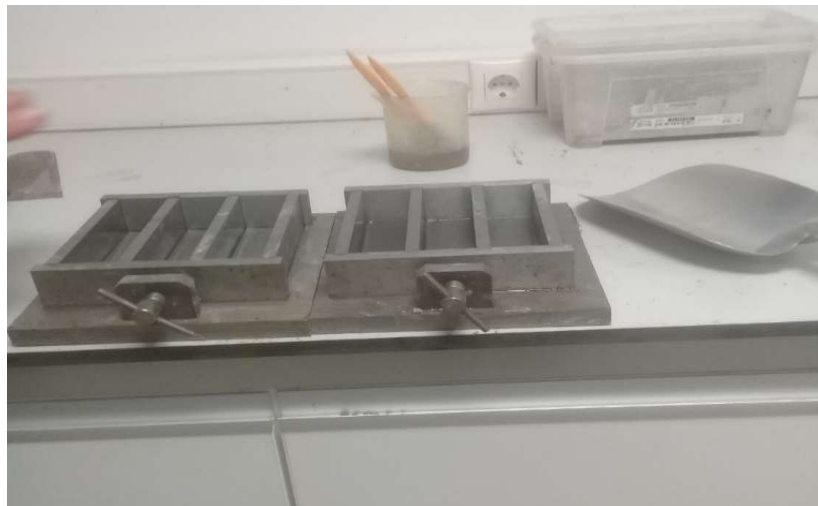
Figure 3 Molds used to make concrete pieces
