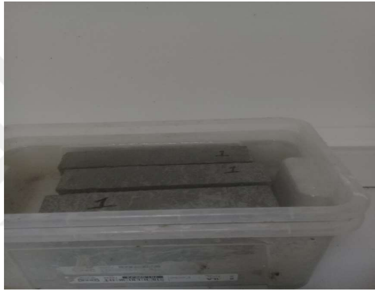
Figure 4 Water tank for concrete pieces
