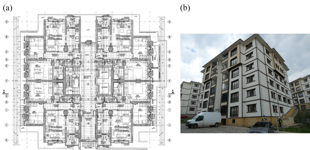
Figure 5. Wall structures with similar amounts of wall in each principal floor plan direction: (a) typical floor plan and (b) example of wall building built by Housing Development Administration of Turkey (TOKI-Toplu Konut Idaresi Başkanlığı) at Dulkadiroglu, Kahramanmaraş.
