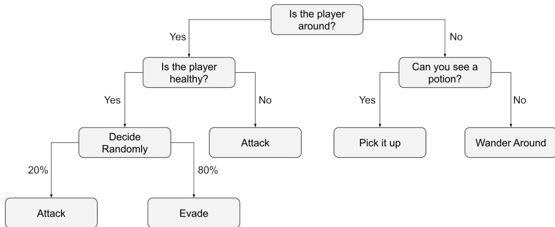
Figure 2: A sample decision tree. If the player is around and healthy, then with a chance of 20 percent, NPC will attack to the player; and with a chance of 80 percent, will evade the player. If the player is not around and the potion is around, then NPC will pick it up.
