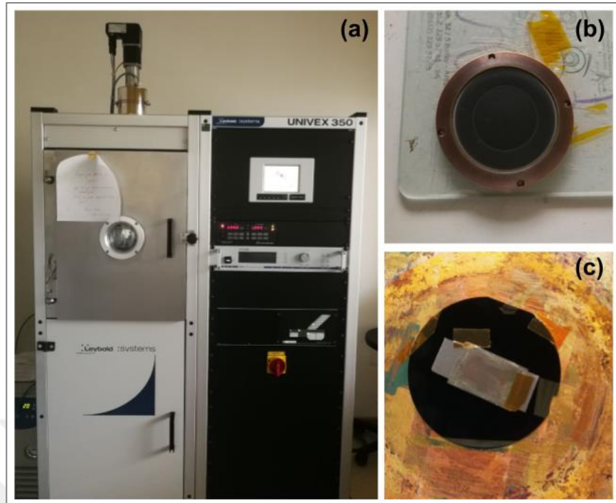
Figure 15. (a) Magnetic sputtering device (Leybold, UNIVEX 350), (b) ITO target, (c) optic lithography applied ITO-PET/Sample 1 fixed on Si with thermal tape.
