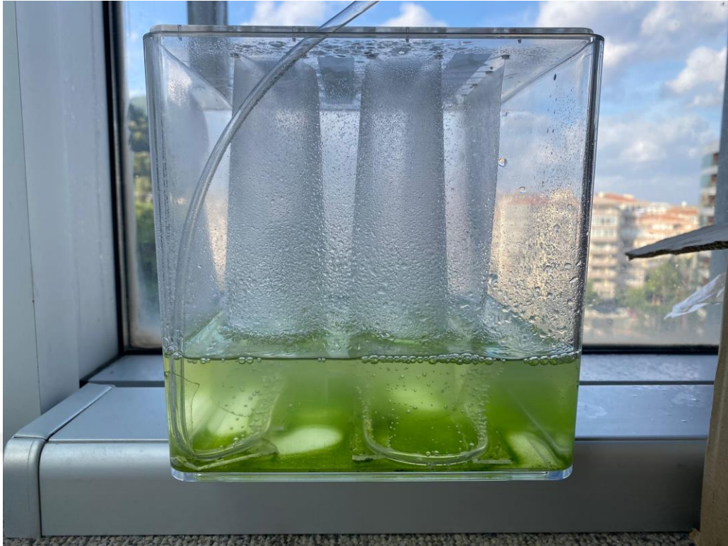
Figure 10. Tank only PBR system at 3 rd floor, south -west façade (prototype 3 at figure 24)
