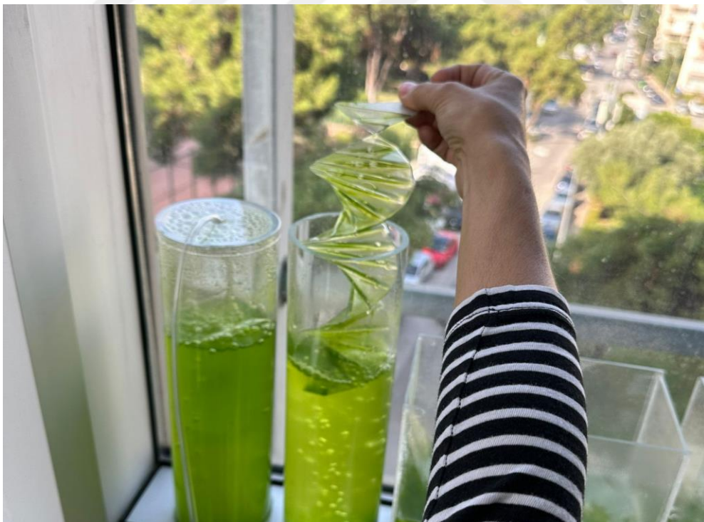
Figure 8. Tubular PBR design spiral sheet added at 3 rd floor, south-west façade (prototype 2 at figure 24)
