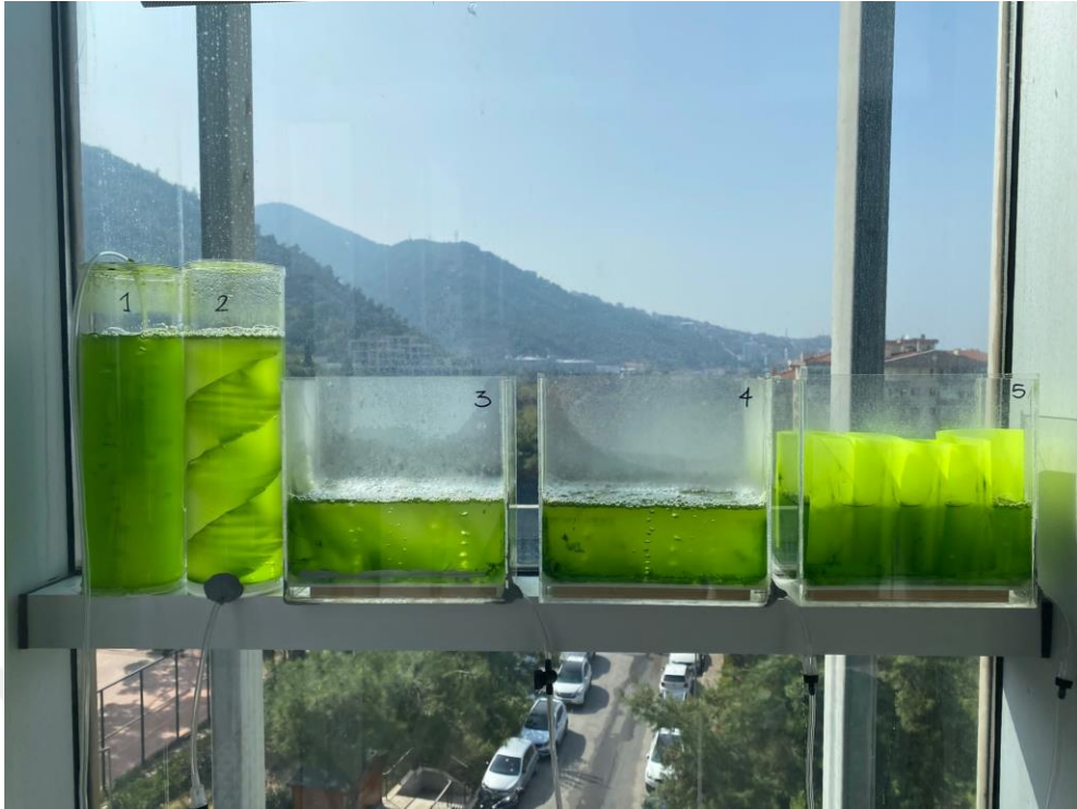
Figure 7. Designed prototypes: 1) donut, 2) spiral, 3) tank with leaf pieces, 4) tank only, 5) tank with “S” shaped PP sheet (prototype 2 at figure 24).
