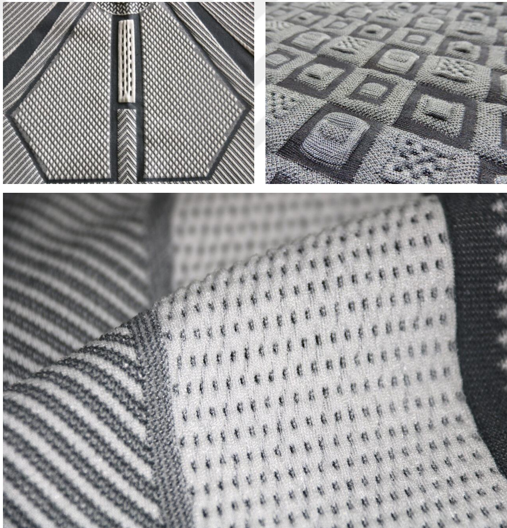
Figure 39. KARL MAYER Piezo-Jacquard Technology/ 3D & 4D Knitting
