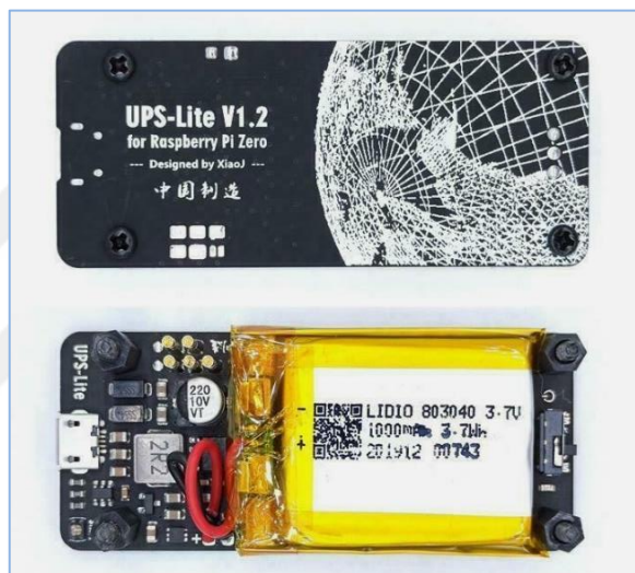
Figure 58. Raspberry Pi Zero 0 W UPS power board
