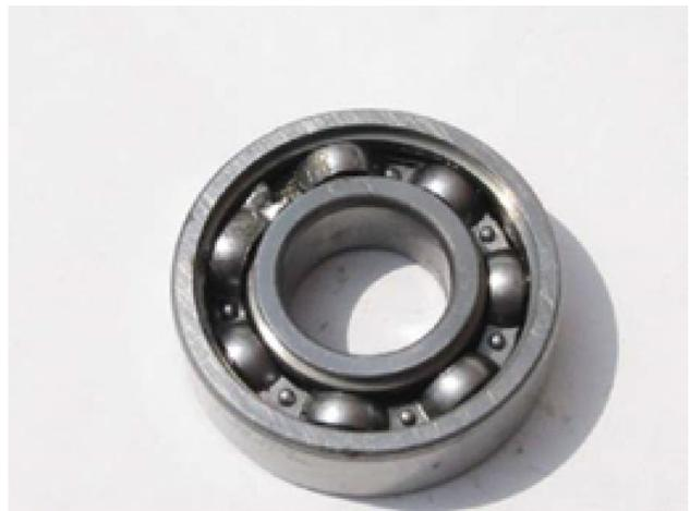
Fig. 4 Cage defect
