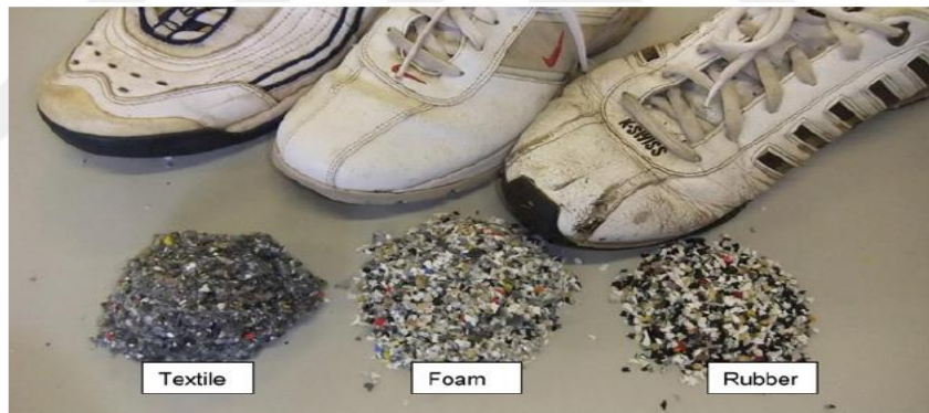
Picture 3.9. Grinding materials such as textile, foam and rubber Source: Staikos and Rahimifard, 2010
