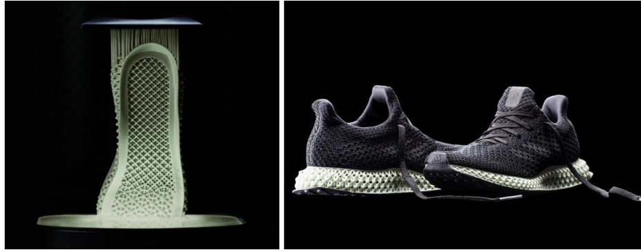
Picture: 3.25. An adidas Futurecraft 4D midsole printing on a Carbon M-series printer to include varying lattice structures along the midsole in one piece Source: https://www.carbon3d.com/stories/adidas/
