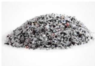
Picture 3.5. Nike Grind Foam; types of midsoles are used Source: Nike, Inc. 2008
