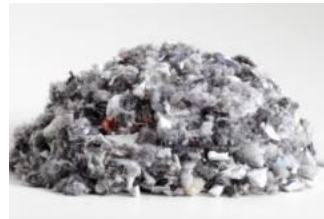
Picture 3.6. Nike Grind Fiber; types of upper parts are used Source: Nike, Inc. 2008
