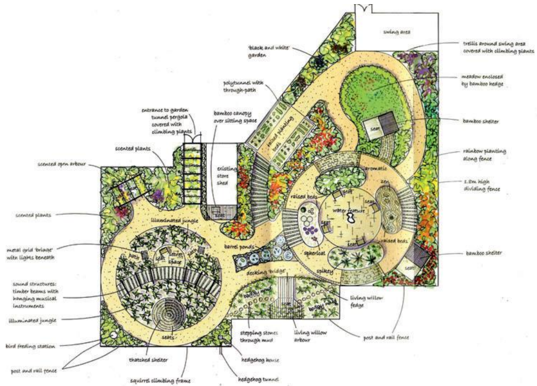
Figure 15. Concept plan of engaging, exploratory sensory garden for mentally disabled residents in mental health village, Buckinghamshire, UK (Souter-Brown, 2014)
