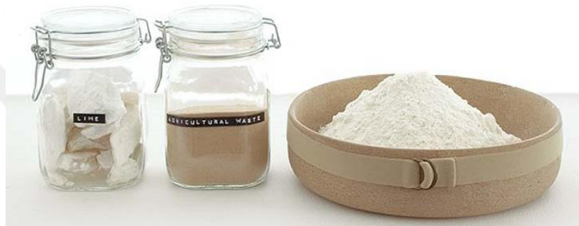
Fig 3.13 Autarchy basic biomaterial ingredients; lime stone, agricultural waste and flour.
