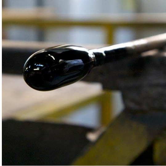
Fig 3.24 Propolis Vessel blow moulding.
