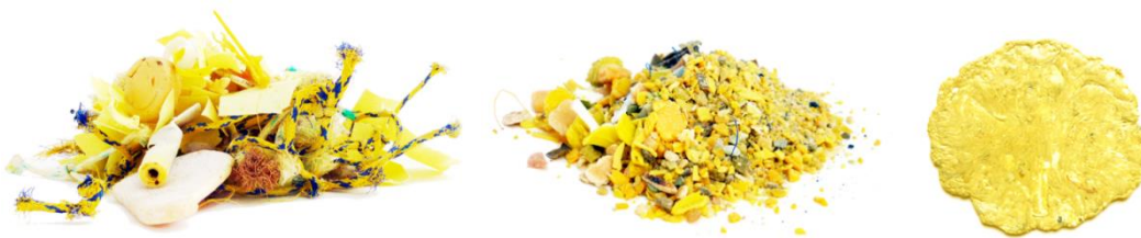
Fig 3.34 Sea Chair's material process; plastic sorting, chipping and melting in furnace. (Source: www.designboom.com )
