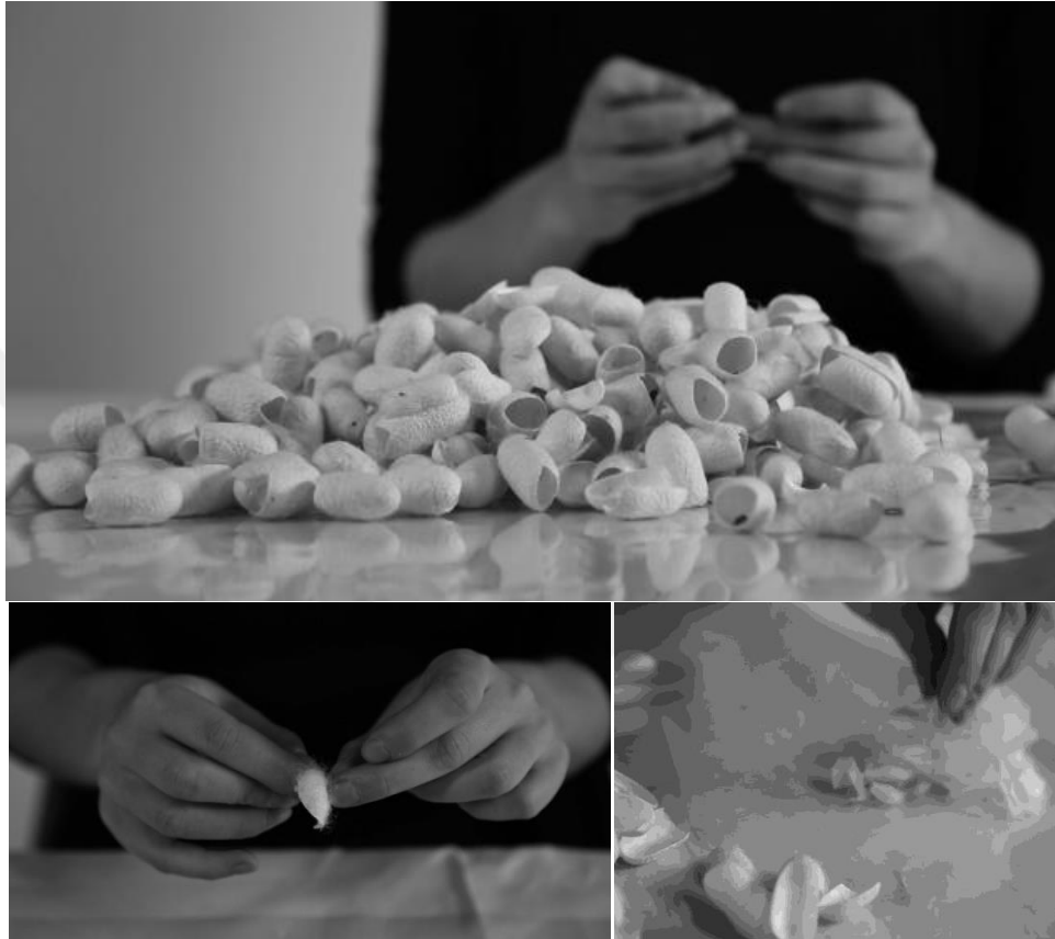
Fig 3.26 Fibre extraction from silkworm cocoons.
