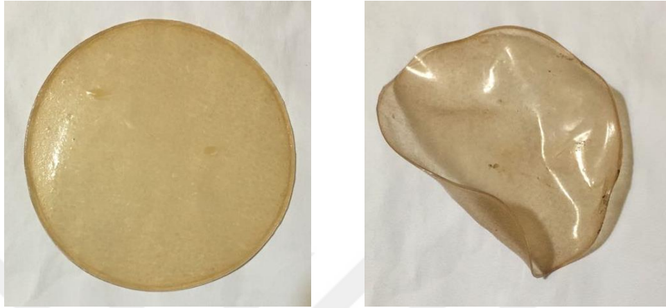
Fig 6.7 Sample 2 left; wet form after water test and right; dried form after the wet form.
