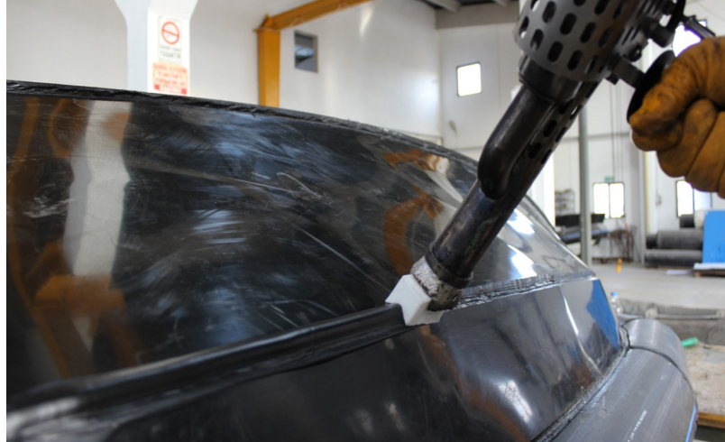
Figure 15. HpdE welding process. Courtesy of, Gözüyılmaz Marine Engineering.
