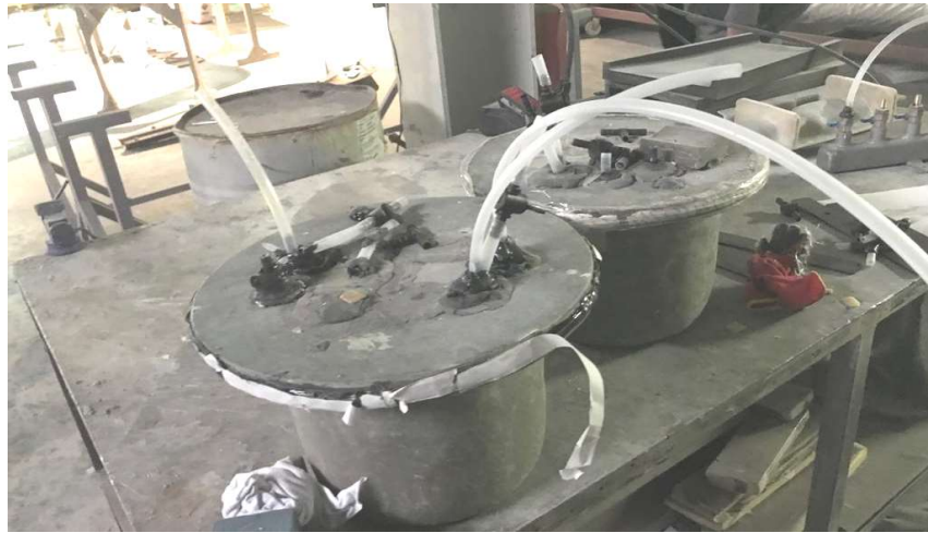
Figure 12. Overflow tank. Courtesy of CSC Composites.
