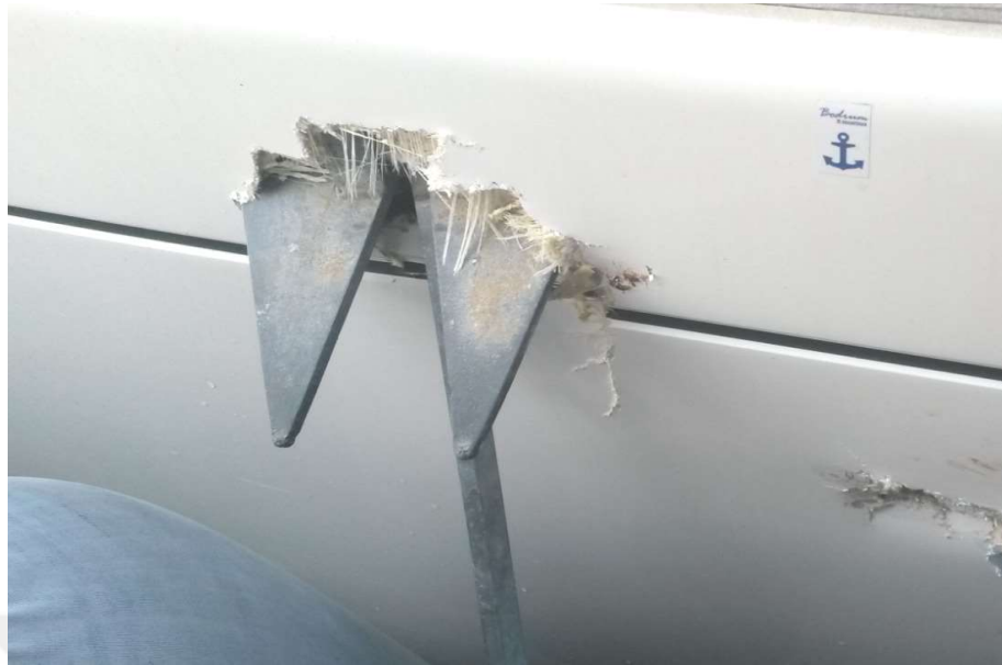
Figure 7. Anchor piercing through the hull. Courtesy of Genco Sindel.
