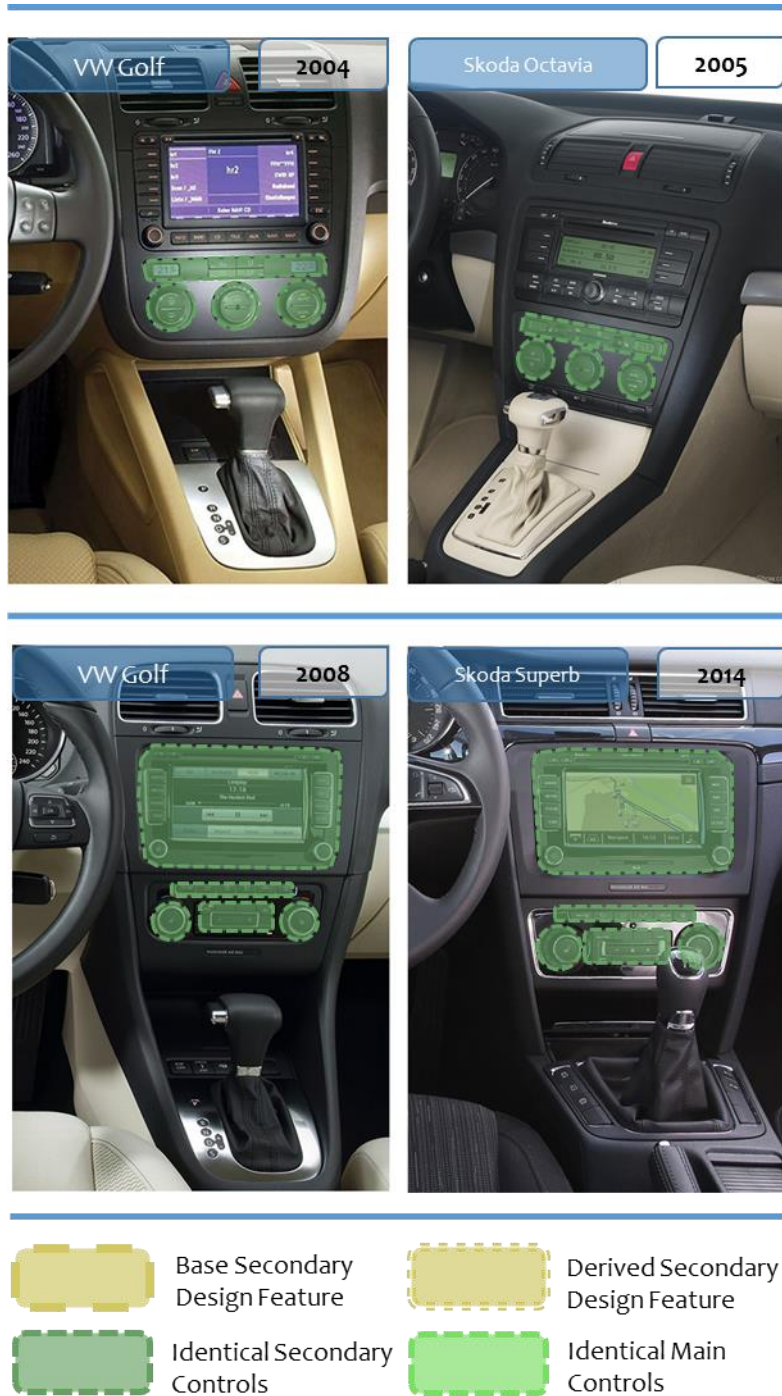
Figure 5.3-4 (continued) Resemblance between Main Control Units, Secondary Control Unit Layouts and Secondary Design Details between Audi, VW Seat and Škoda Products (NetCarShow, n.d.)
