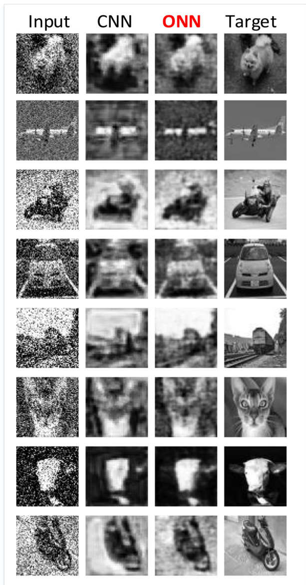
Fig. 13 Some random original (target) and noisy (images) and the corresponding outputs of the best CNN and ONN from the test partition
