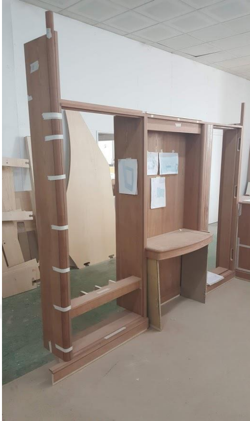
Figure 38. Cabinet Unit & Makeup Table for the Master Cabin Area
