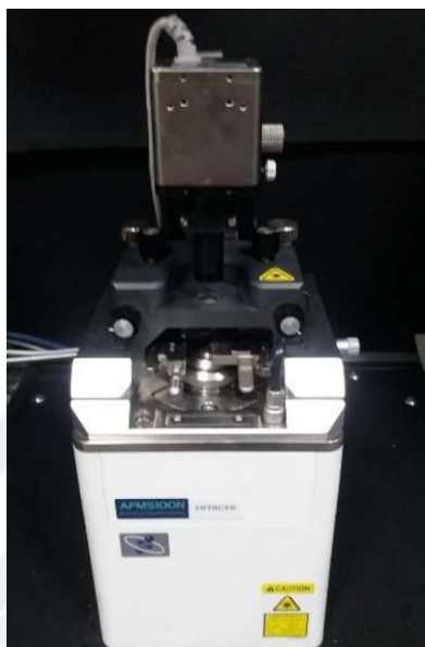
Figure 15. Hitachi multifunction SPM unit AFM 5100N
