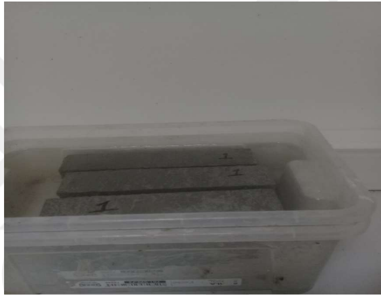
Figure 4 Water tank for concrete pieces
