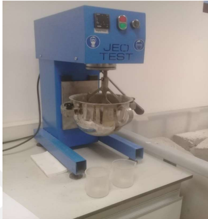
Figure 2 Mixer used for mixing the materials
