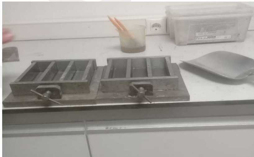
Figure 3 Molds used to make concrete pieces
