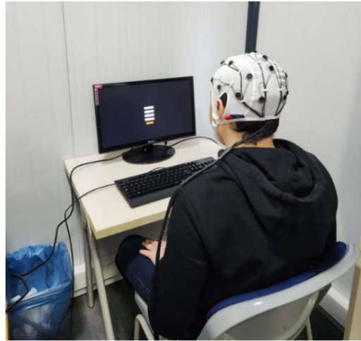
Figure 1. Motor imagery EEG experiment setup showing a participant with an OpenBCI EEG cap interacting with the Unity-based stimulus interface.
