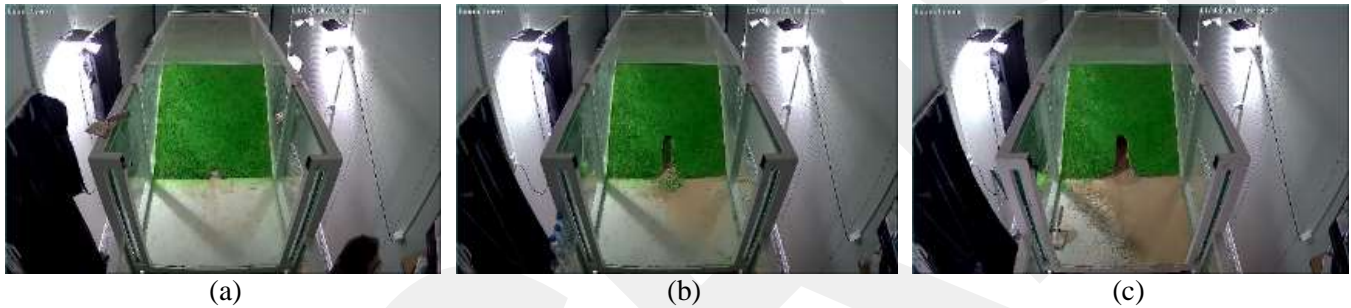
Fig. 6: The temporal development of the breach at downstream a) t=0\text{ h} , b) t=48\text{ h} , c) t=230\text{ h}
